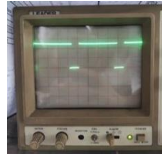
Figure 10. PWM signal generated with 20V input voltage
