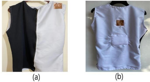
Fig. 19. Jacket and two antennas on (a) Front side, (b) Back side
