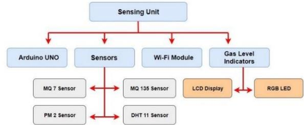
Figure 3: Components of the sensing unit Sensors
