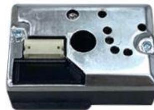
Figure 5: Sharp GP2Y1014AU0F Sensor
