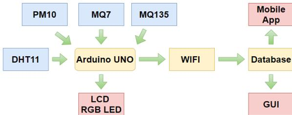
Figure 2: Overall IoT system with WSN
