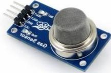
Figure 6: MQ 7 Gas Sensor
